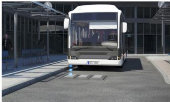
Figure 9 Floor mounted ACD Alstom solution
