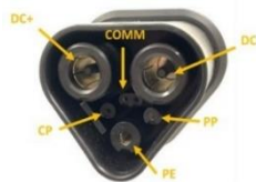
Figure 4 Megawatt Charging Plug Layout
