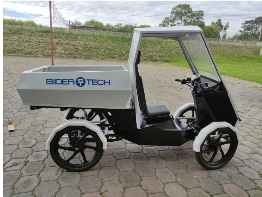
Fig 2. Prototype of quadricycle (Phoenix) developed by SIDERTECH
