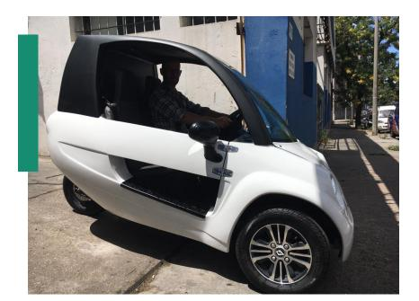
GreenStar SRL is an SME that produce electric three-wheelers composed of a steel framed chassis and a fiber glass body. The powertrain was originally acquired in China. Their markets are the local market (Uruguay) and they are also working to allocate their product in the USA.
