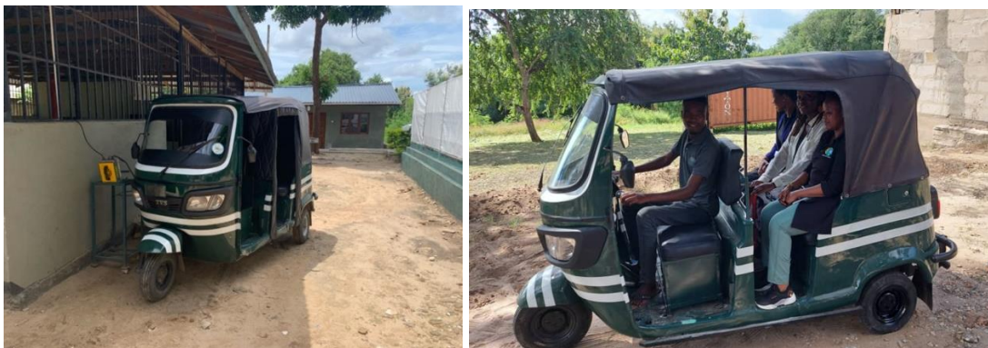
Figure 12. Three retrofitted ICE three-wheelers by SESCOM (Martin, 2024; Owigar, 2024)
