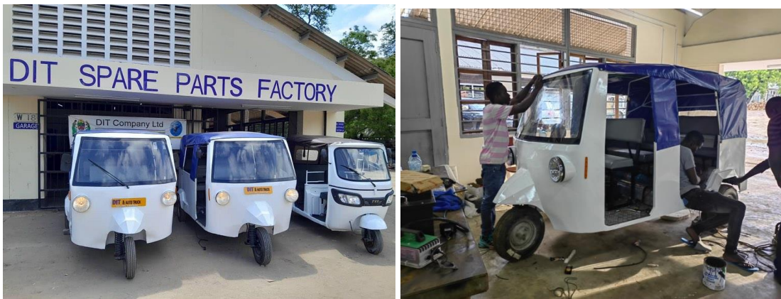
Figure 11. One retrofitted ICE three-wheelers and two new e-three-wheeled prototypes by Auto Truck and DIT Company Ltd (Martin, 2024; DIT, 2023)
