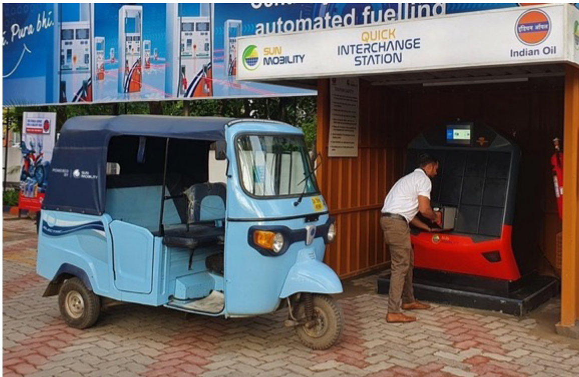
Figure 20. Electric three-wheeler at a battery swapping facility in Chandigarh, India (Ranjan, 2020)
