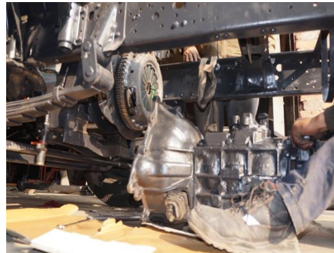
Motor fitted to chassis, coupling with the gear box
