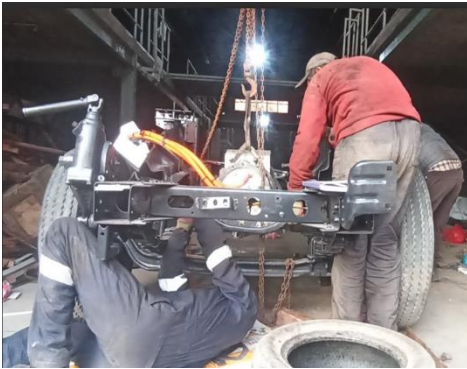
Replacing engine with motor
