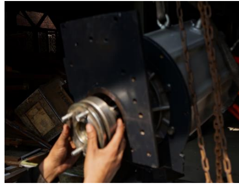
Fixing roller bearing on the motor shaft
