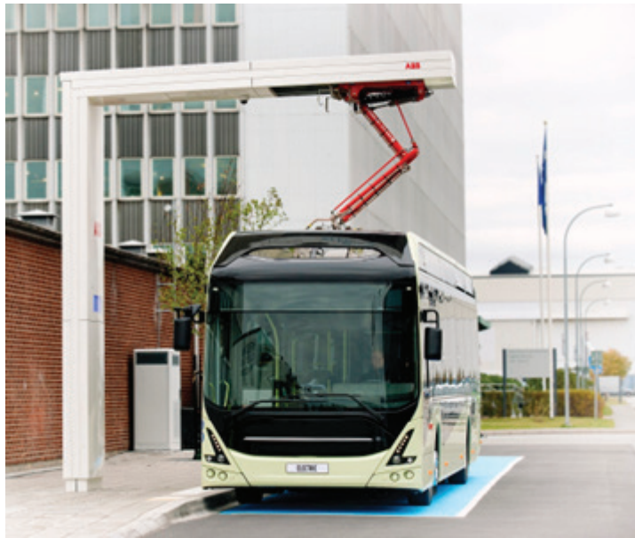
Figure 13: e-Bus charged with inverted pantograph technology (source: new.abb.com)
