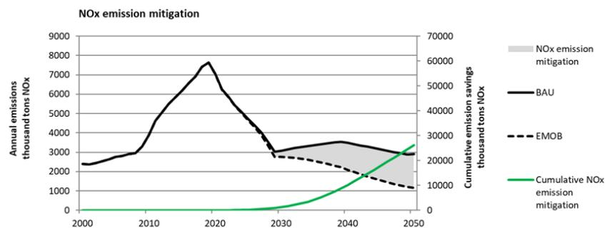
Figure 10. NOx emission mitigation for e-bajaj scenario
