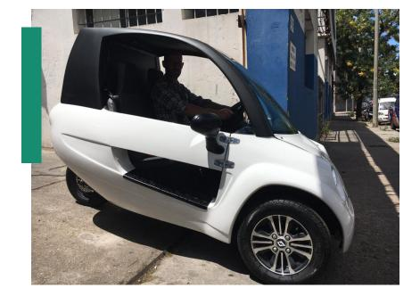
GreenStar SRL is an SME that produce electric three-wheelers composed of a steel framed chassis and a fiber glass body. The powertrain was originally acquired in China. Their markets are the local market (Uruguay) and they are also working to allocate their product in the USA.
