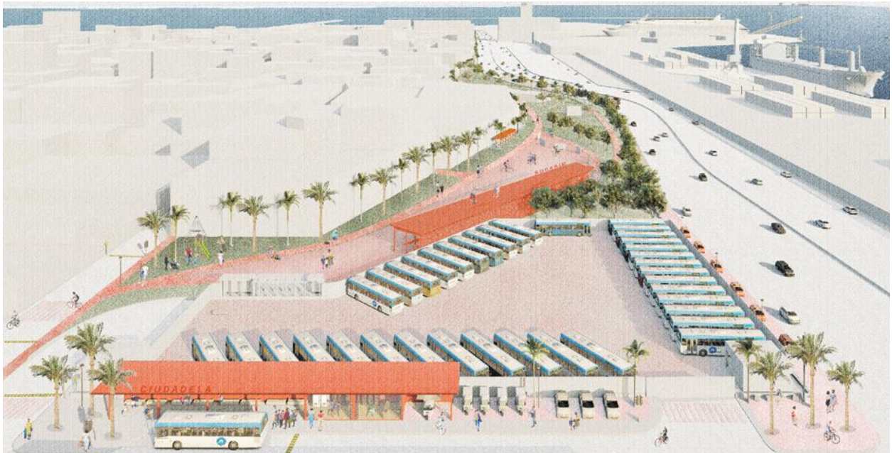
Figure 7 - North view of the Terminal with the proposal for the location of different types of vehicles, chargers and infrastructure intervention. (Source: Design studio of TUB).
