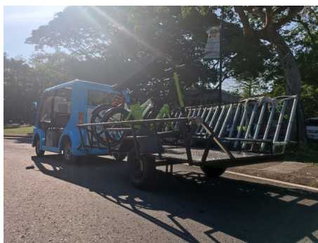
Figure 4 SOLplus Equad serves as a redistribution vehicle for the shared mobility scheme at the UPLB Campus
