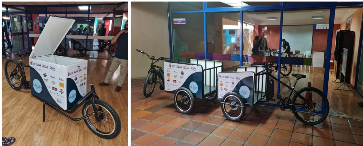
Fig 3. Locally assembled e-cargo bikes, long john type (left), rear-load and front-load tricycles (right)
