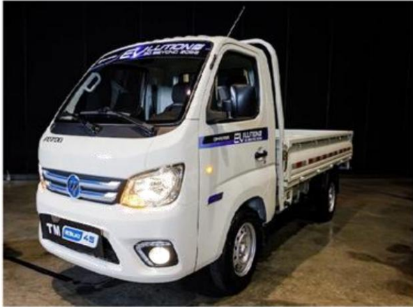
Truck mate TM iBlue45 Battery 44.9 kWh Driving range 275 km/charge Motor 75 kW
