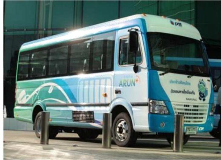
Truck mate TM iBlue45 Battery 44.9 kWh Driving range 275 km/charge Motor 75 kW
